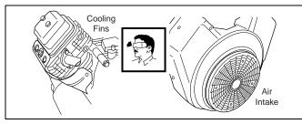
Fig. 36 Cleaning Air Intake and Cooling Fins
